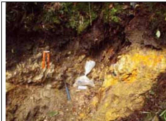
Channel sampling of weathered and altered feldspathic tuff (Suarez Fm) with limonite-haematite staining derived from sulphides
