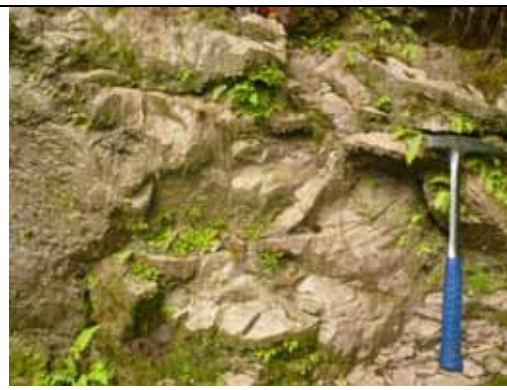
Medium grained feldspathic tuff (Suarez Fm) with pervasive argillic and silica alteration characteristic of epithermal type mineralization
